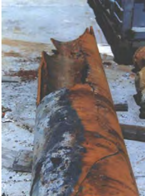
Pitting and Fatigue leading to Pipe Failure - Ductile Iron
