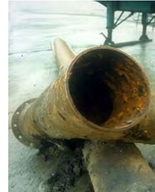
Corrosion Inside the Pipe
