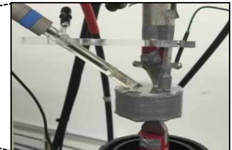
Electrochemical corrosion cell made of plexiglass
