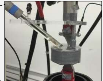
Electrochemical corrosion cell made of plexiglass
