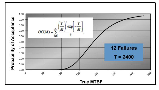
M = true but unknown reliability of the system and c = maximum number of allowable failures T = total demonstration test length
